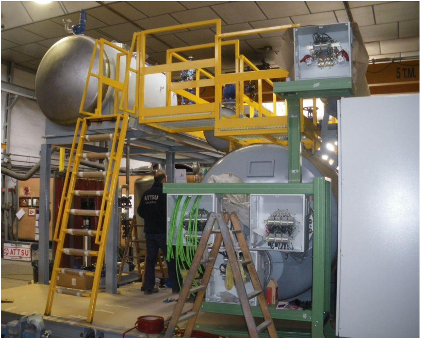
GE-2400 WITH SUPERHEATER – IN THE PROCESS OF MANUFACTURE
